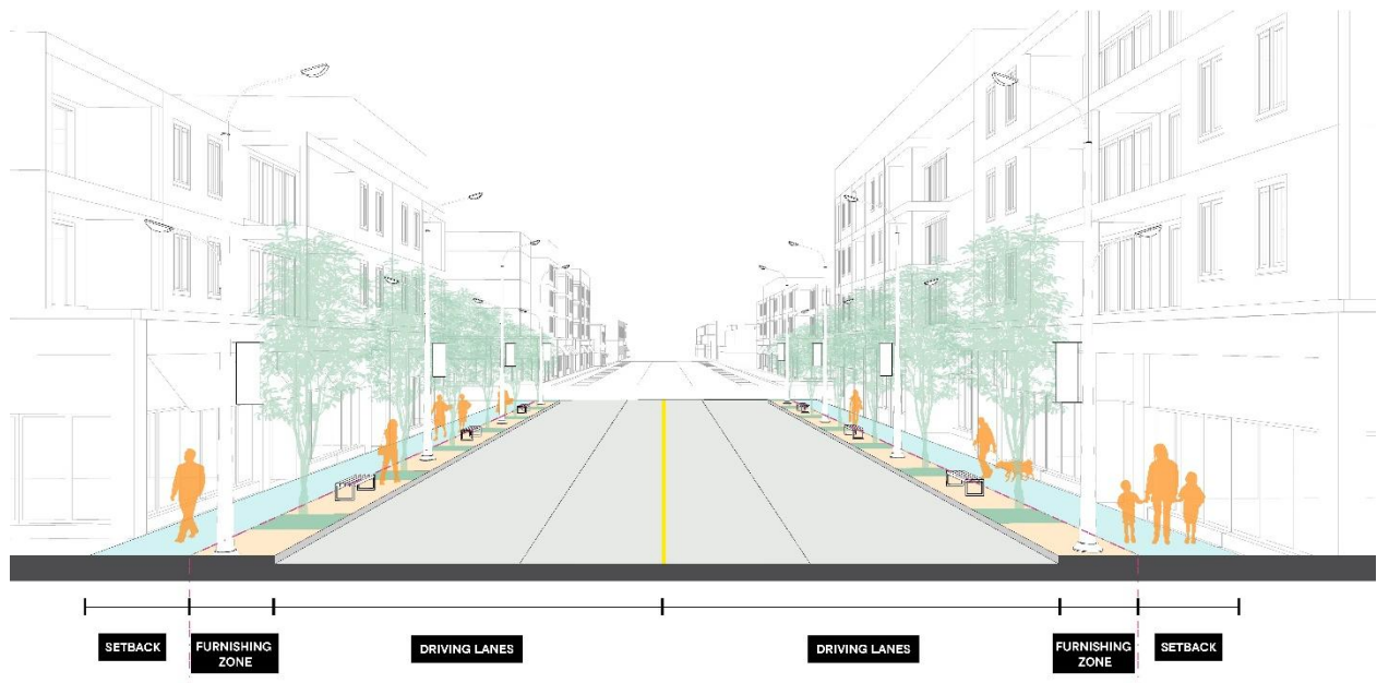
Figure 2: Example Arterial Section with Constrained Right-of-Way
