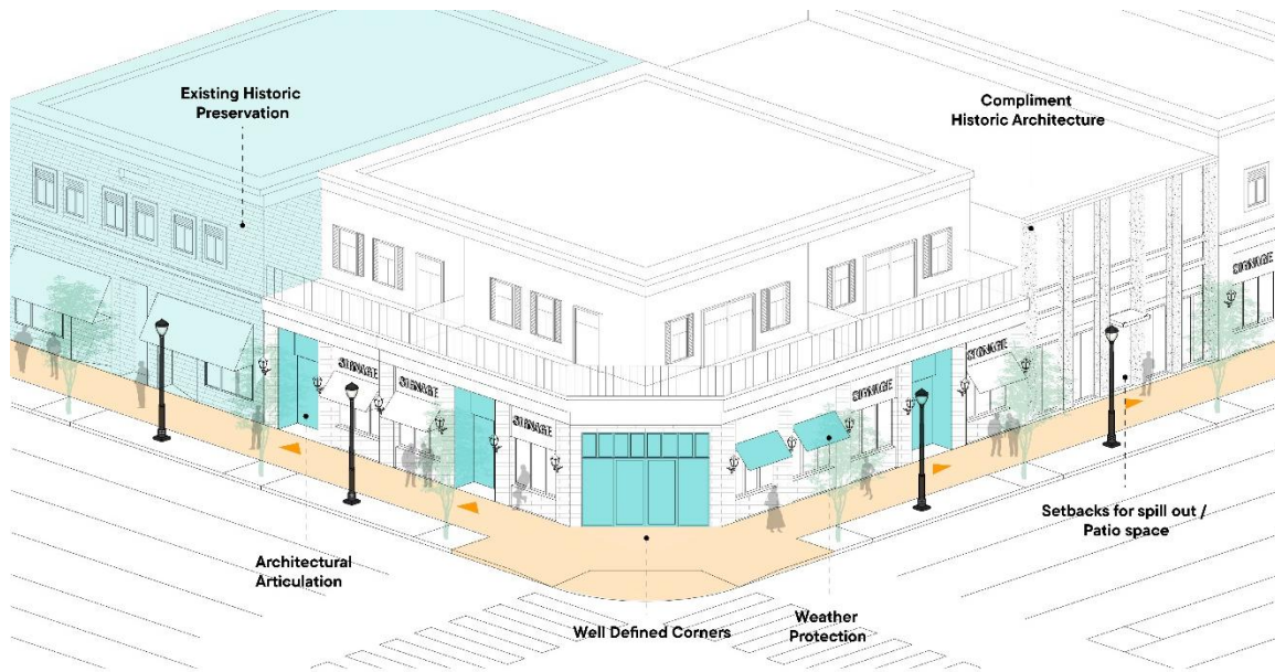
Figure 14: Historic Main Street Character and Street Interface
